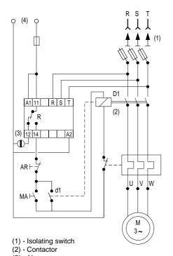
Monitoring of three-phase motor. Manual re-engage after disappearance of the
