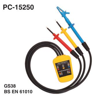
A fast, effective method of identifying worn or unmarked cables, and ensuring all 3-phase outlets and machinery are wired correctly. The PC15250 will also quickly and simply prove continuity of all three lines, or identify which are faulty as well as showing the sequence of phase rotation.
