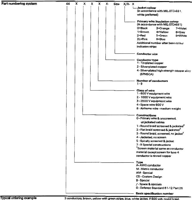
3 conductors, brown, yellow with green strips, blue, white jacket. If 600 volt, round braid. 20 AWG tinned conductor, total part number is 44A1131-20-1/45/6-9.
