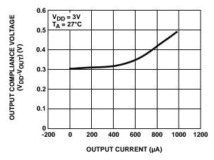
FIGURE 7. OUTPUT COMPLIANCE VOLTAGE vs CURRENT
