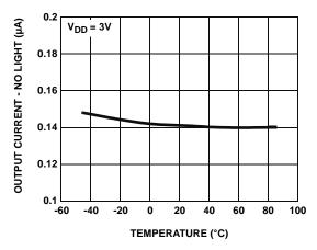
FIGURE 5. DARK CURRENT vs TEMPERATURE
