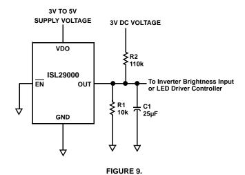
Next the value of R $_2$  can be calculated based on the maximum output current coming from the ISL29000 under the application's maximum light exposure. Suppose the current has been determined to be about 125 $\mu$ A. Thus R $_2$  can be calculated approximately as follows:
