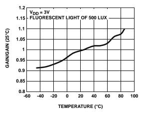
FIGURE 6. GAIN vs TEMPERATURE
