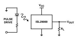
FIGURE 1. RISE/FALL TIME MEASUREMENT
