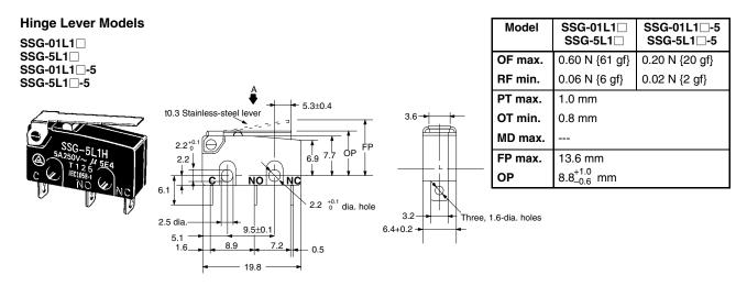
Note: Also available are models with a hinge lever length of 39 mm under the following model numbers; SSG-01L14, SSG-5L14, SSG-01L14, SSG-01L14
