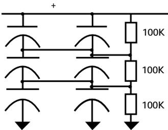
The two resistors are used to ensure that the leakage currents of the capacitors does not affect the circuit reliability, by ensuring that all the capacitors have half the working voltage across them.
