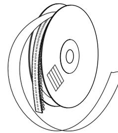
Holding tape outside. Positive terminal leading (negative terminal by special request).
