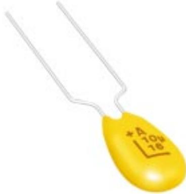
TAP is a professional grade device manufactured with a flame retardant coating and featuring low leakage current and impedance, very small physical sizes and exceptional temperature stability. It is designed and conditioned to operate to +125°C (see page 27 for voltage derating above 85°C) and is available loose or taped and reeled for auto insertion. The 15 case sizes with wide capacitance and working voltage ranges means the TAP can accommodate almost any application.
