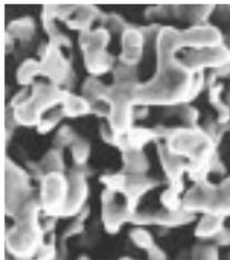
This is subsequently vacuum sintered at high temperature (typically 1500 - 2000°C). This helps to drive off any impurities within the powder by migration to the surface.
