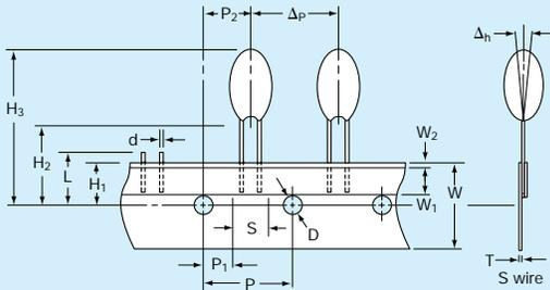
'S' and 'D' wire for special applications, automatic insertion on 2.5mm pitch.
