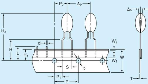
'B' wires for normal automatic insertion on 5mm pitch.
