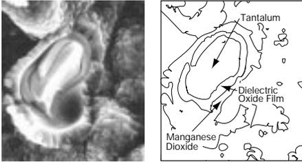
The next stage is the production of the cathode plate. This is achieved by pyrolysis of Manganese Nitrate into Manganese Dioxide.
