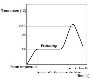
Note: The above curve is given on condition that the thickness of the PCB is 1.6 mm.
