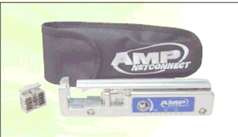
The built in jacket stripper makes cable preparation clean and fast (no fumbling for a separate cutter) while the lacing fixture is extremely simple to use - it has a cable clamp that holds the cable in place while all eight of the conductors are laced into the wire positioning slots, making sure the conductors stay in place during the termination process.
