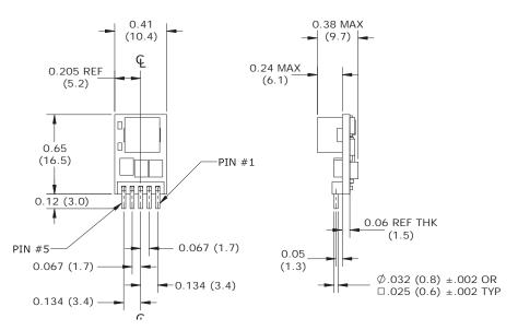
Figure 2 . LSS-T/10-W12 Series Component locations are typical.
