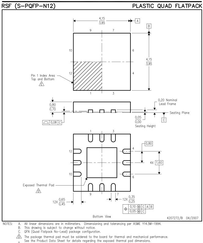
Pin 1 identifiers are located on both top and bottom of the package and within the zone indicated. The Pin 1 identifiers are either a molded, marked, or metal feature.
