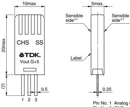
Pin No. 1 Analog output voltage Pin No. 2 GND
