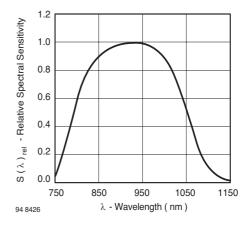
Figure 6. Relative Spectral Sensitivity vs. Wavelength
