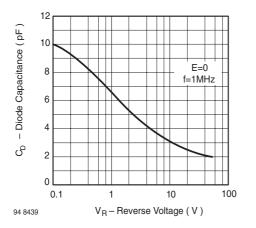
Figure 5. Diode Capacitance vs. Reverse Voltage
