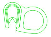
fit metal adhesion widht 1-4mm
