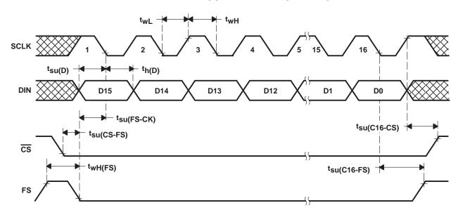
Figure 1. Timing Diagram
