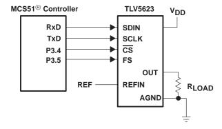
Figure 18. TLV5623 to MCS51® Controller Interface
