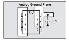
Figure 20. Power-Supply Bypassing
