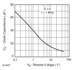
Figure 6. Diode Capacitance vs. Reverse Voltage
