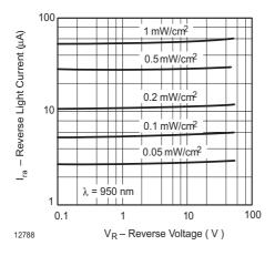
Figure 5. Reverse Light Current vs. Reverse Voltage
