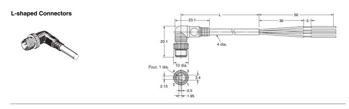
S8 Snap-in Connectors with Vibration-proof Robot Cable
