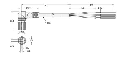
S8 Snap-in Connectors with Vibration-proof Robot Cable
