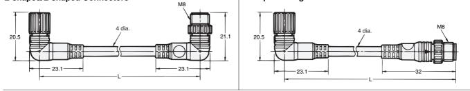
S8 Snap-in Connectors with Vibration-proof Robot Cable
