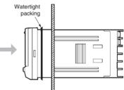
**3.** Insert the adapter into the grooves on the left and right sides of the rear case and push until it reaches the panel and is fixed in place.
