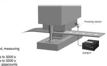
Inputs: Passing speed, cycle, time difference, time band, measuring length, interval
