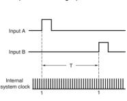
The time (T) between input A pulse and input B pulse is measured by the internal system clock. If, for example, the system clock measures 100,000 counts during time T, then
