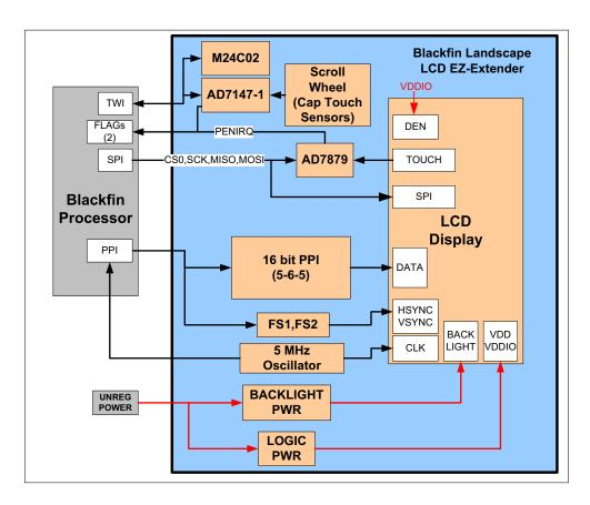
Figure 2-1. Block Diagram
