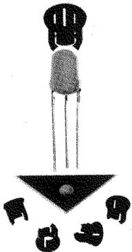
Designed for use with T-1 & T-1 3/4 LED's in .060 - .070 thick panels. The holder snaps into the front panel with easy, light-finger pressure. The LED snaps into the holder from behind the panel and is held securely in place.
