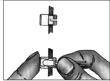
Designed for use with T-1 or T-1 3/4 LEDs, these Lens Caps are available in round or square configurations. They snap-mount through the front panel for easy, light-finger pressure, installation. The LED is inserted into the cap from behind the panel and held securely in place.
