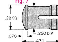
\*When mounting T-1 3/4 Low Profile Caps (Fig. 4 or Fig. 7) in panels .125 thick or less a spacer must be used. Spacer CAT. NO. 8692 MATERIAL: White Nylon 3.8 O.D. x 1/4 I.D. x 1/8 Lg.
