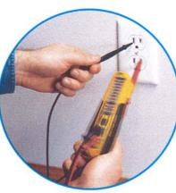
Vibration mode gives a tactile indication of the voltage level.
