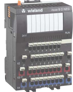
Binary I/O module 24 V DC 8 outputs, negative switching
