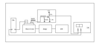
SG: Programmable Signal Source HP 8165A Amp: Power Amplifier Exciter: Exciter B&K 4809 Acc: Accelerometer B&K 8309 DUT: Device (FS-2513P) under test CA: Charging Amplifier B&K 2635 IA: Impedance Analyzer HP4192
