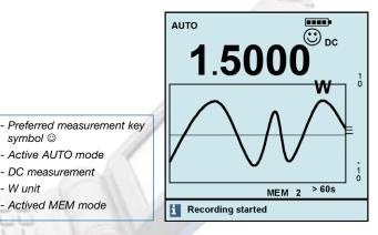
Thanks to technological improvements resulting in a single "A" terminal, current measurements may be carried out from a single switch position, making for fluid and trouble-free changes of the measurement range, from just a few hundred micro Amperes to up to 20 Amperes.
