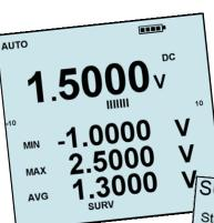
In addition, its **SURV** function enables you to display and record simultaneously the minimum, maximum and average values of a given measurement, as well as the date/time recording of limit and beginning and end values, for the period monitored.
