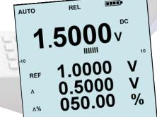
Thanks to the instrument's 4 digital displays, the relative function **REL** provides comprehensive simultaneous display of the absolute and absolute drift values, relative drift % and reference value. For greater comfort, the reference value can be adjusted directly using the **REL** function key.
