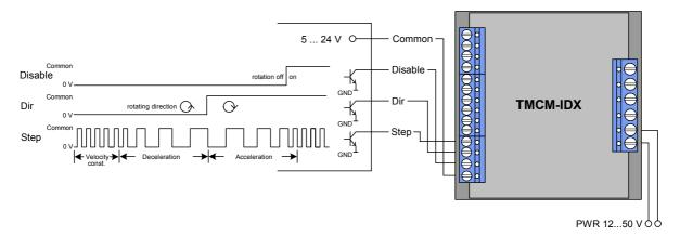
Figure 5.3: Contacts for Step-Direction
