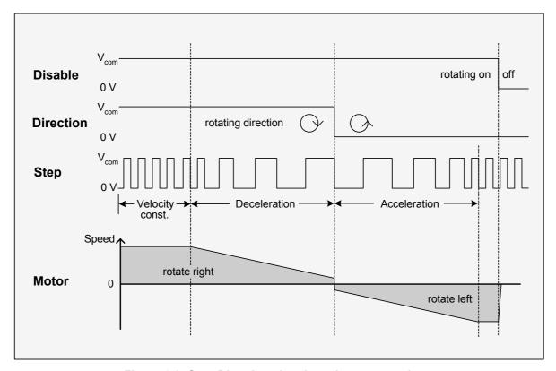
Figure 6.2: Step-Direction signals and motor reactions
