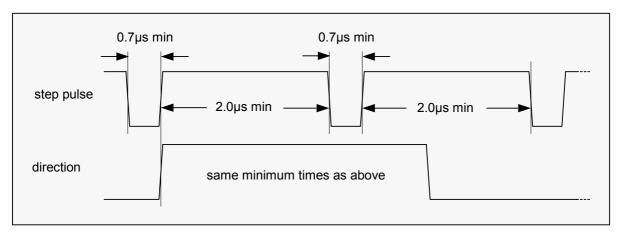
Figure 6.3: Step and Direction Signal
