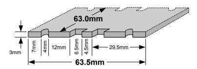
Figure 3.3: Base Plate Dimensions
