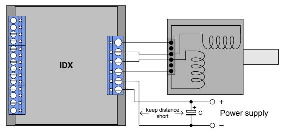
Figure 5.2: Connecting Motor and Power Supply
