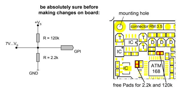
Figure 6.7: Layout Changes for DC-Motor option
