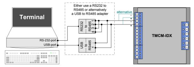
Figure 5.4: Contacts for RS485 with an adapter
