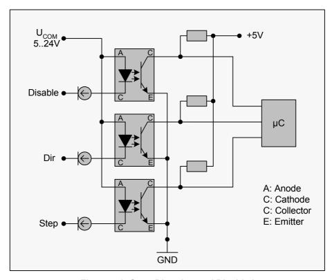
Figure 4.1: Step, Direction and Disable Inputs
