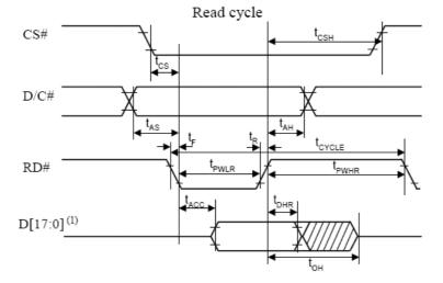
8080-series MPU parallel interface characteristics
