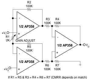
$V_0 = (1 + \frac{2R_2}{R_1})(V_2 - V_1)$
