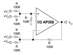
Where:  $V_0 = V_1 + V_2 - V_3 - V_4$  $(V_1 + V_2) > (V_3 + V_4)$  to keep  $V_0 > 0$   $V_{DC}$
