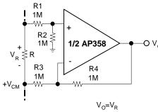
Ground Referencing a Differential Input Signal
