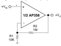
\*R not needed due to temperature independent I<sub>IN</sub>
