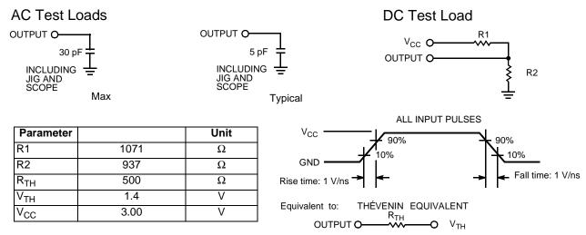
Figure 12-7. AC Test Loads and Waveforms for Digital Pins
