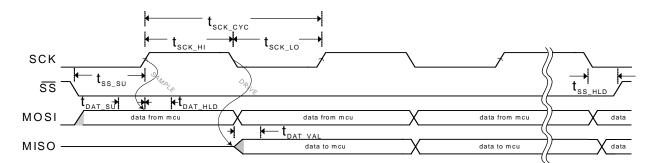
Figure 12-1. SPI Timing Diagram
