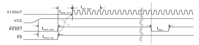
Figure 12-5. Power On Reset/Reset Timing
