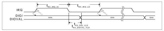
Figure 12-3. DIO Receive Timing Diagram
