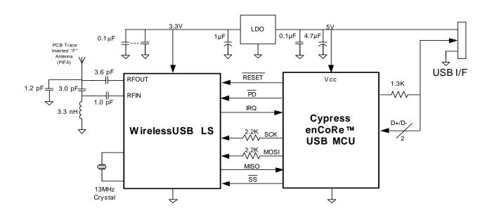
Figure 6-2. CYWUSB6934 USB Bridge Transceiver
