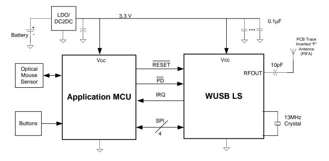
Figure 6-1. CYWUSB6932 Transmit-Only Battery-Powered Device
