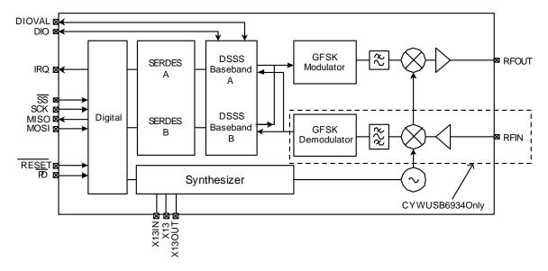
Figure 3-1. CYWUSB6932/CYWUSB6934 Simplified Block Diagram
