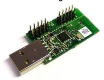
A reference design for a CC1111/CC2511 based full-speed USB dongle with RF interface. Should be used as reference design for antenna and RF layout.
