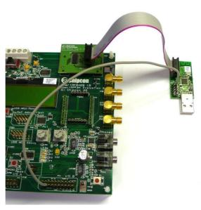
Figure 3. USB Dongle Powered from SmartRF04EB
