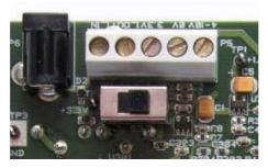
Figure 4. SmartRF04EB Power Switch, Power On
