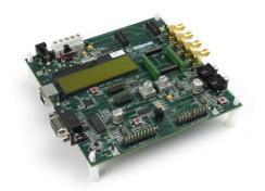
Evaluation Board. Main board in the development kits, USB interface, LCD, LEDs, pot-meter etc. Development platform for the Evaluation Modules (EM).
