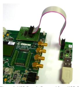
Figure 2. USB Dongle Powered from USB Cable
