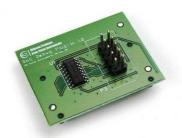
The System-on-Chip Debug Plug-In Board. It provides an additional physical debug/programming interface for the SmartRF04EB. Referred to as SOC\_DEM in this document.
