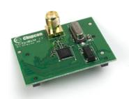
CC1110 and CC2510 Evaluation Module are small modules for the CC1110 and CC2510 devices. These can be plugged into the SmartRF04EB and they should be used as the reference design for antenna and RF layout.
