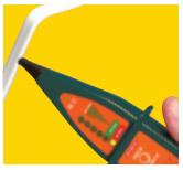
BROKEN WIRE - 1 LIGHT READING AND AUDIBLE ALERT
