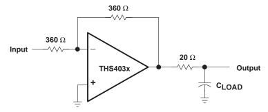
Figure 49. Driving a Capacitive Load
