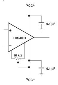
Figure 50. Offset Nulling Schematic
