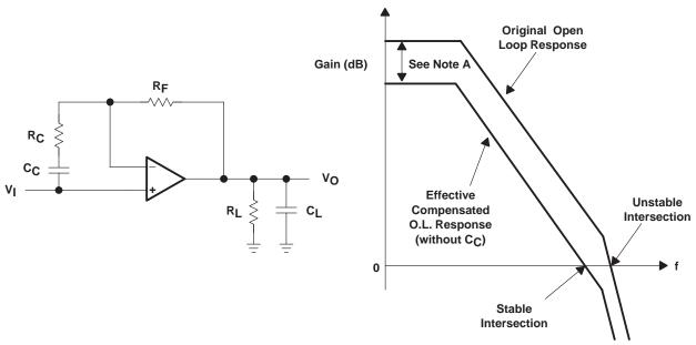
NOTE A: The difference is due to 1+R<sub>F</sub>/R<sub>C</sub> noise gain.
