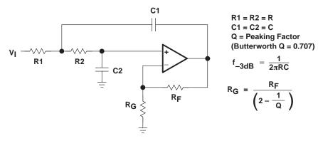
Figure 53. 2-Pole Low-Pass Sallen-Key Filter
