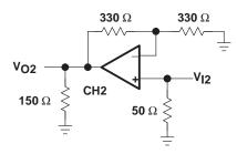
Figure 3. THS4032 Crosstalk Test Circuit
