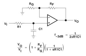
Figure 52. Single-Pole Low-Pass Filter
