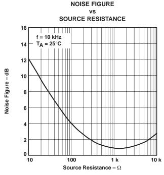
Figure 45. Noise Figure vs Source Resistance
