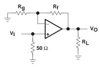
Figure 4. Step Response Test Circuit
