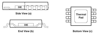
NOTE B: The thermal pad is electrically isolated from all terminals in the package.
