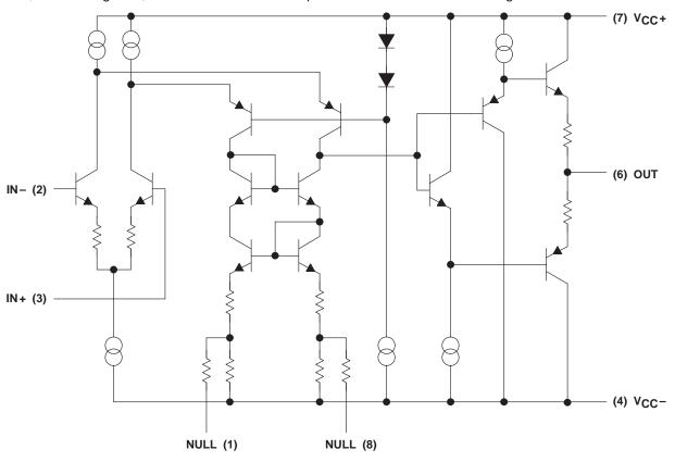
Figure 43. THS4031 Simplified Schematic
