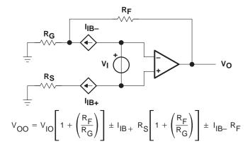
Figure 51. Output Offset Voltage Model
