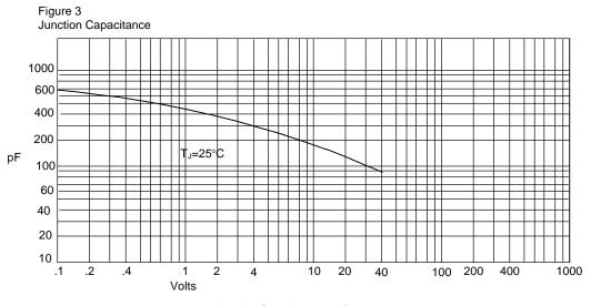
Junction Capacitance - pFversus Reverse Voltage - Volts
