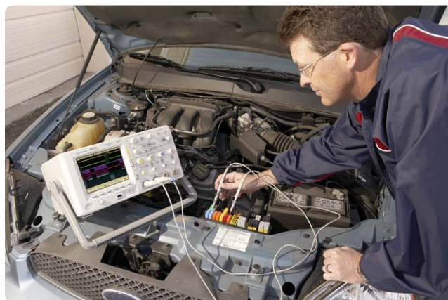
Figure 9. Making remote CAN and LIN measurements with Agilent's battery option for InfiniiVision Series scopes.
