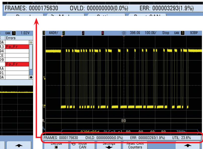
Figure 2. Real-time totalize functions provide CAN bus efficiency and quality measurement statistics.
