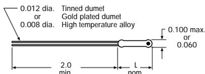
VECO® Bead-In-Glass Probes consist of bead thermistors with sintered-in platinum-iridium leads embedded in solid glass. Hermetically sealed, they have excellent stability over long periods of time under continuous exposure to harsh environments. They retain excellent stability at temperatures to 325°C (617°F) for storage or continuous operation, and to 550°C (1,022°F) for intermittent operation. For complete product information request VECO Bulletin MGR061.
