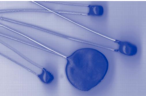
VECO® Military Grade general purpose chip and disk style thermistors meet the requirements of MIL-PRF-23648. They are designed for temperature measurement, control, or compensation applications within a temperature range of -55°C to + 125°C. Both disc and chip styles exhibit excellent long-term stability. The disc style is available in either ratio, A or B, and the RTH44 chip style is available in ratio B only. See Technical Bulletin MMT103.
