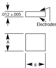
**Easily Mounts Directly Onto Substrate.** These new thermistors are available in a wide range of resistances (with up to 1% tolerance) and feature top/bottom metalization for easy mounting on substrate. Designed to meet MIL-PRF-23648 and MIL-STD-883; standard contact surface is silver. VECO® Surface Mount Thermistors are also available with gold or palladium/silver contacts. For special attachment requirements, see Product Bulletin FP-0071.
