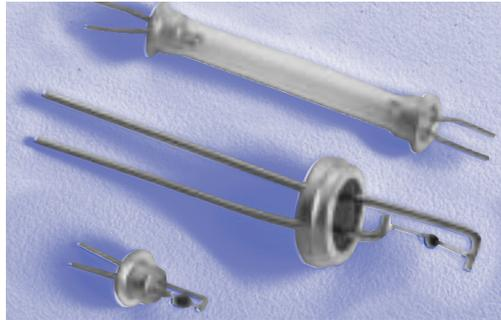
VECO® bead thermistors utilize metallic oxide semiconductor material sintered on platinum-iridium alloy lead wires and feature a hermetic seal via a controlled glass coating for excellent stability under continuous exposure to conductive, corrosive, and other hostile environments. Fast response times and high power sensitivities in a mini size make them
