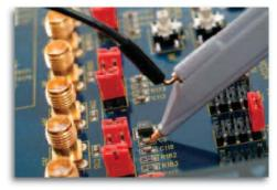
A variety of standard and available probe tip and grounding accessories are offered to meet any requirement. What's more, ZS Series probes are available for a very affordable price. Use the ZS1000 with 200 and 600 MHz WaveSurfers and the ZS1500 with 1 GHz WaveSurfers to give full system bandwidth at the probe tip.
