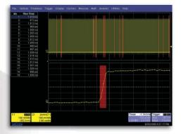
**Mixed Signal Oscilloscope Option** Add 32 digital channels to a 4-channel WaveSurfer Xs with the MS-32 Mixed Signal Oscilloscope option. Includes 32 Mpts of digital memory (1 Mpts/Ch) for long capture times.
