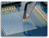
1 and 1.5 GHz active probes with 0.9 pF, 1 M $\Omega$  input impedance and an extensive probe tip and ground accessory selection.
