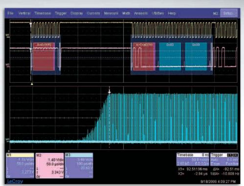
in the EEPROM. It can also aid in monitoring DATA outputs from I<sup>2</sup>C-based sensors, such as analog-to-digital converters, and triggering when DATA is outside a safe operating range. In both cases, verifying proper operation becomes a simple task.
