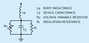
Figure 2. TransGuard Equivalent Model.
