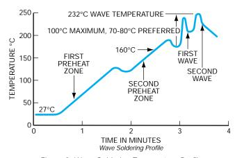
Figure 3: Wave Soldering Temperature Profile
