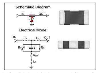
but the roll-off characteristic becomes much flatter, resulting in EMI filtering over a much broader frequency spectrum. Typical applications include filtering/protection on Microcontroller I/O Lines, Interface I/O Lines, Power Line Conditioning and Power Regulation.
