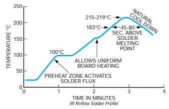
Figure 2: Infrared Reflow Temperature Profile
