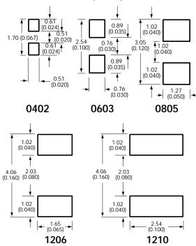
Figure 1: TransGuard Solder Pad Dimensions
