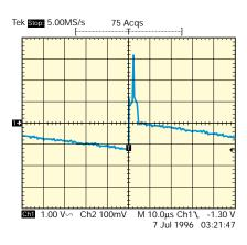
Fig. 5A. 24 V Relay Transient with 26 V TransGuard 10 V/Division
