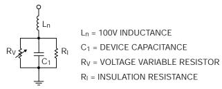
Figure 4. Antenna Varistor
