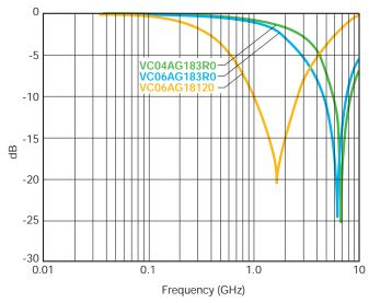
Figure 5. Attenuation vs Frequency
