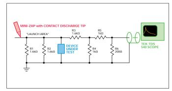
Figure 2. Schematic of Test Set Up
