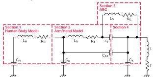
Where: C<sub>H</sub> = Lumped capacitance between the human body and earth
