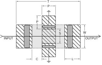
Note: It is only necessary to ground one center terminal. However, AVX recommends that both side terminals be connected.
