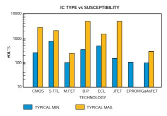
Figure 3. IC Type E Field Susceptibility
