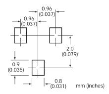
Figure 1B. SOT23 - Solder Pad Layout
