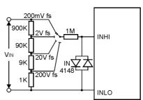
For multi-range, use, a 2 pole, 4 way rotary switch. 1 pole for range select and the other to connect the appropriate decimal point to V+
