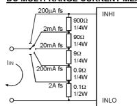
For multi-range, use, a 2 pole, 5 way rotary switch. 1 pole for range select and the other to connect the appropriate decimal point to V+
