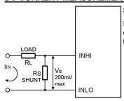
Shunt resistance  $Rs = \frac{Vs}{IIN} \Omega$
