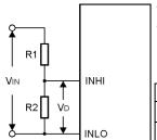
To measure voltages greater than 200mV an attenuator is required.
