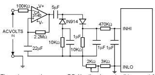
The meter can only measure DC. Use the above circuit to convert AC to DC. For voltages above 200mV AC, a potential divider is required before the converter circuit as shown in the "Voltage measurement" section above
