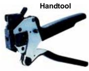
Hirose offers tooling to suite all production volumes. Hand tooling conveniently allows termination on site or in the factory environment, whilst the T12 press & applicator only requires mains electricity and lends itself to high volume production in the factory. Both tools terminate the plugs in one
