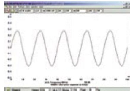
Equivalent Time Sampling (ETS) boosts the 100 MS/s sampling rate of the ADC-212/100 to a staggering 5 GS/s for repetitive signals.
