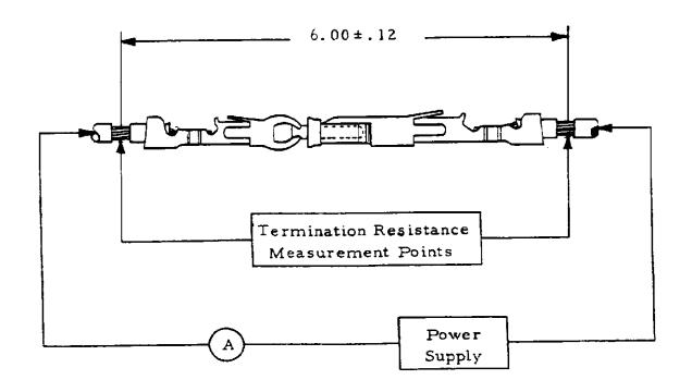
NOTE: Termination resistance equals millivolts divided by test current less resistance of 4.5 inches of wire
