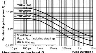
Maximum pulse load Pi, max. for continuous pulses
