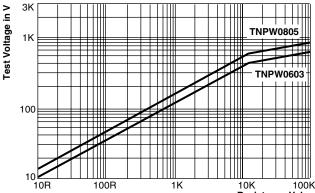
Single-Pulse High Voltage Overload Resistance Value in O Test 10/700 µs EN140000 4.27
