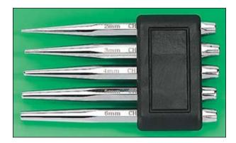
Material: Base- PE Punch-CR-V6150 + Chrome finished. Hardness of the punch: 52~55HRC Size of the punch: 2 x 120mm 3 x 120mm 4 x 120mm 5 x 120mm 6 x 120mm Content: 1set/box Package: 60sets/ctn, 0.48'/18/19KGS
