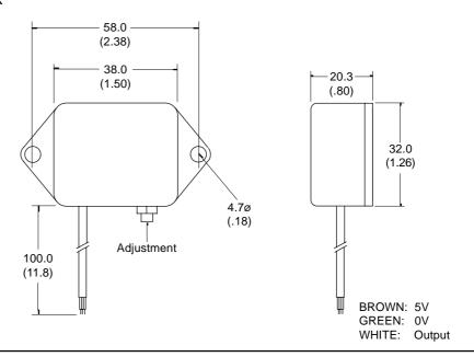
This sealed tilt sensor has a differential angle of 15°. The output signals are logic levels with a degree of de-bouncing applied. The ammount of debounce is adjustable via a potentiometer. The output signal can be used to drive a transistor if required.
