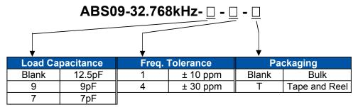
\*Contact ABRACON for non-standard load capacitance
