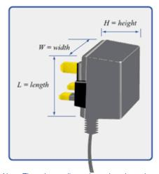
Note: The adaptor dimensions given here do not include the plug pins and mounting plate of the plug-top model shown
