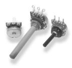
A popular range of 20mm control potentiometers, the type 23 series can be tailored to suit more specific requirements. The potentiometers are available with printed carbon resistance element, choice of bush lengths in metal or plastic and insulated shafts up to 50mm in length. In addition, approved mains and low current switches are available as standard options.
