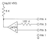
Figure 2 Sensing Bridge Supply Circuit
