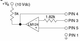
Figure 2. Sensing Bridge Supply Circuit
