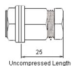
To accommodate cable diameters 7.0 to 10.5mm
