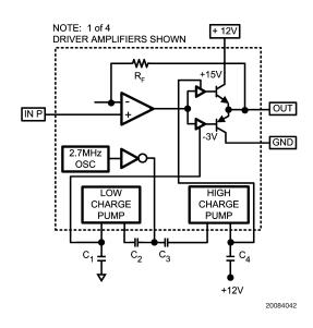
FIGURE 2. Internal Connections of Integrated Charge Pumps
