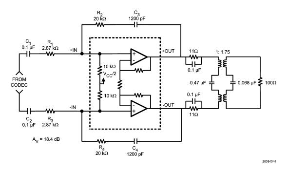
FIGURE 4. MTPR Measurement Test Circuit
