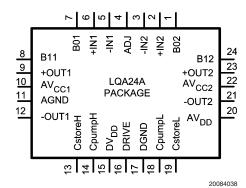
Note: Die attach pad is electrically connected to AGND
