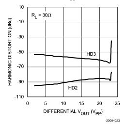
Harmonic Distortion @  $I_{CC}$  = 11.4 mA, 1 MHz
