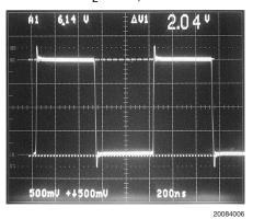
Large Signal Pulse Response @  $R_L = 36\Omega$ , 1 MHz
