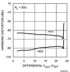
Harmonic Distortion @ I<sub>CC</sub> = 16 mA, 1 MHz
