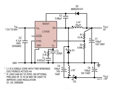
Figure 14. Dual Output SEPIC Converter
