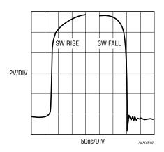
Figure 7. Switch Node Resonance
