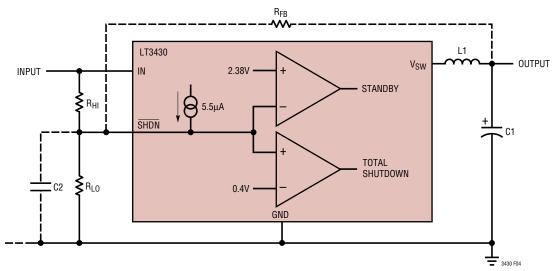
Figure 4. Undervoltage Lockout
