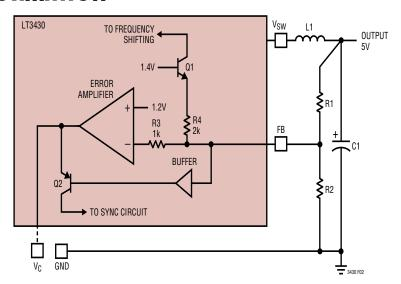
Figure 2. Frequency and Current Limit Foldback
