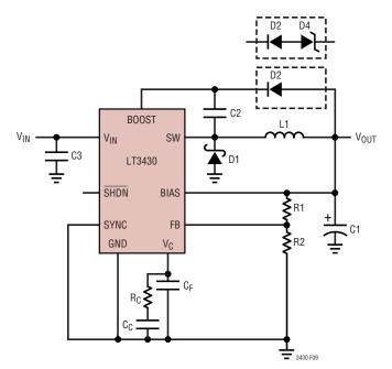
Figure 9. BOOST Pin. Diode Selection
