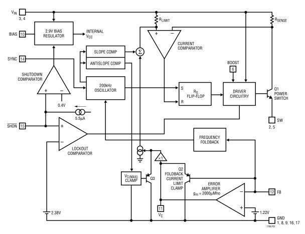
Figure 1. LT3430 Block Diagram
