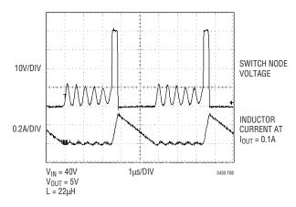
Figure 8. Discontinuous Mode Ringing
