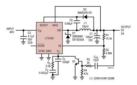
Figure 13. Buck Converter with Adjustable Soft-Start
