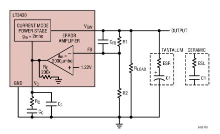
Figure 10. Model for Loop Response
