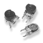
This tiny 6mm square cermet trimmer is offered with alternative adjustment covers for screwdriver and automatic setting and can be supplied in bulk or taped in ammo pack. The 416 can be adjusted from the top or side and is an inexpensive solution to high reliability potentiometer requirements. This series is used to replace some of the larger, expensive, sealed types in high volume circuits.
